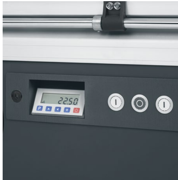
Height and tilt displayed digitally on an LCD monitor.
