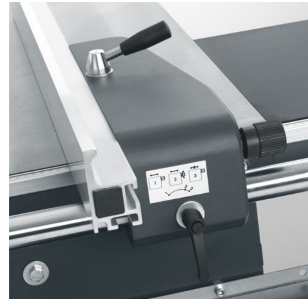
Rip fence with precise manual adjustment.
