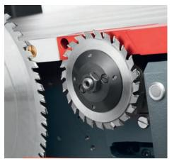
**Parking position:** The new unit allows the scorer to be moved out of the working area to a much better protected standby position, allowing it to be "parked" safely out of the way when processing solid wood, plastic materials or even aluminium.
