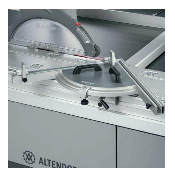
**DUPLEX double-sided mitre fence.** DUPLEX fences enable bevel cuts at any angle between 0 and 90° with speed and precision. Set it to 45° and a mitre cut can be made on both sides of the workpiece without further adjustments. Dimensions of the flip stops are set using a measuring scale and magnifier. All DUPLEX fences can be positioned anywhere along the entire length of the table. With no more than 17 kg all DUPLEX models now have improved handling.
