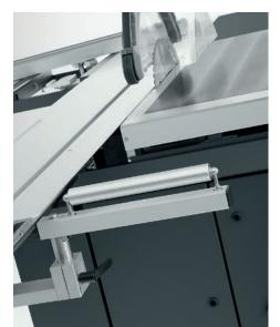
**Front support roller.** The 300 mm-wide front support roller is particularly useful when cutting longer workpieces on the rip fence. It can be folded down through 90° in one movement to stow under the sliding table (minimum length 3,000 mm) when not required.
