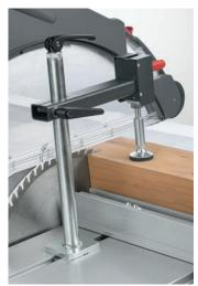
**Manual quick-action clamp.** The alternative to the pneumatic quick-action clamp. The manual quick-action clamp can be easily positioned on the sliding table and fixed. The workpiece is then firmly secured on the table and the crosscut fence. It has a clamping height of up to 200 mm and provides extra safety at very little extra cost. Not available in CE region.
