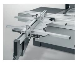
**DIGIT LD:** for 1/10mm accuracy when setting the length dimension. The display shows all stop settings applied. The central measuring and display unit calibrates the entire system in one operation and angles are displayed in digital format, enabling a level of precision of  $\pm 1/100^{\circ}$ . The length dimension is calculated automatically as a function of the mitre angle. Two flip stops with fine adjustment, two batteries and a charger are included.
