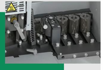
**PUR Box:** Our PUR box slows down the hardening of PUR adhesive in glue pots by using a compressed air drying process, increasing the potential processing time of the adhesive up to 7 days before cleaning is required. This accessory is recommended if regularly working with PUR adhesives.
