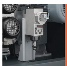
Changeable motor for corner rounding: The preset interchangeable motor including tool allocation reduces machine set-up time when changing the front head radius. The quick-change preliminary setup allows the motor to be changed quickly without the need for any additional settings.
