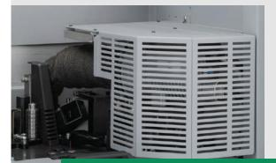
**AirTronic:** Joint-free appearance using hot air technology. Easily switch between EVA, PUR or AirTronic in your edge banding machine without the need for tools and effortless perfect your finished result. Pre coated edges are symbolically "fused" with your panel materials by means of a high-temperature nozzle to create a homogenous surface that leaves nothing to be desired. This takes just 3 minutes to heat up and only requires changing the edge channel.
