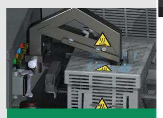
Automatic glue pot refilling system: A large storage tank for up to 5 kg of granules ensures maximum efficiency. The glue pots are filled automatically so that even high cycle times can be easily handled without the need for manual filling.
