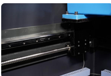
Backgauge use ball screw and linear guide rail
